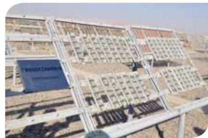
▶ Xin Jiang Testing Center(Continental Desert Climate)Temperature: -28°C to 50°C Highest Land temperature: 70°C
